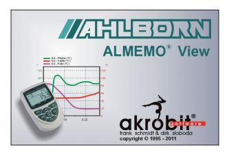
**ALMEMO®** View is a software package that can be used to evaluate and display measured data on any ALMEMO® device with 2 or 3 measuring inputs.
